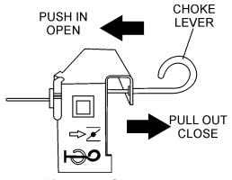
Figure 11. Choke Lever
